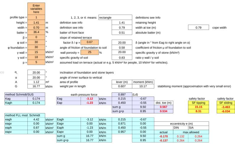
Spreadsheet for calculating earth pressure force, sliding and tipping values of retaining wall profiles.
